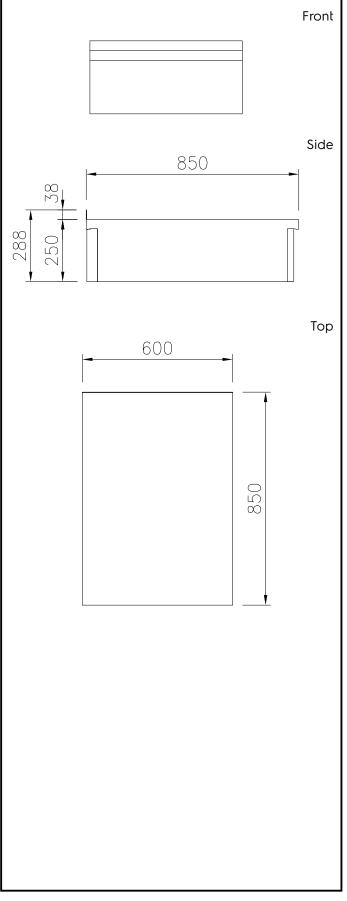
Modular Cooking Range Line thermaline 85 - 600 mm Closed Work top, 1 Side with Backsplash
